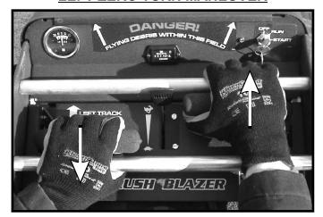
Grab the left steering control handle with your left hand and pull back while at the same time grabbing the right steering control handle with your right hand and pushing forward. This will spin the machine left, without mowing forward.
